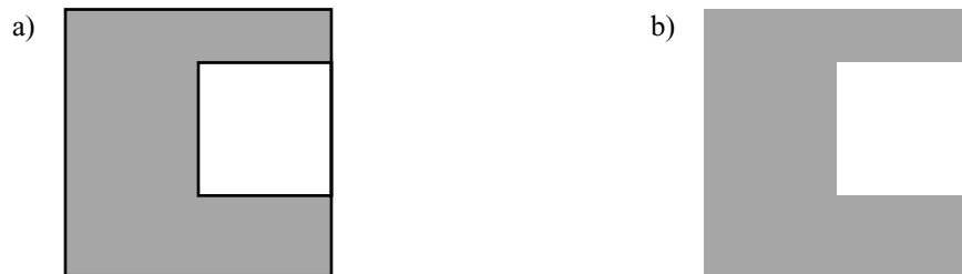
Figure 2-2: A simple HSBM object with node outlines (a), and without node outlines (b)
